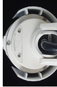
External SD card slot with cover (Add rubber for waterproof)
