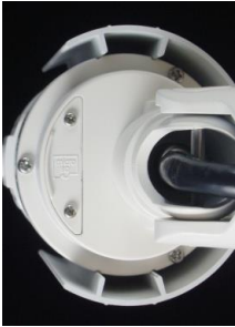
External SD card slot with cover
