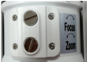
External zoom / Focus adjustment
